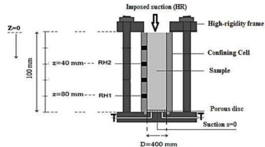
Fig. 2. Permeameter test to determine the unsaturated permeability of intact soil sample
