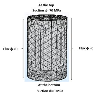
**Fig. 3.** Tridimensional mesh used in the numerical computing and boundary conditions.
